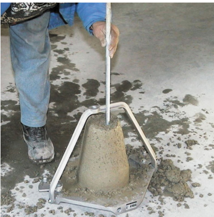
54-C0149/B slump cone kit during operation. The handle raises over specimen and slump is measured using the tamping rod engraved in 1 cm increments.
